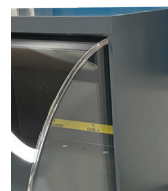
PVC safety enclosure for testing up to 15 kVAC
