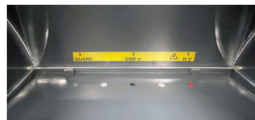
Connection to internal terminals of the device under test
