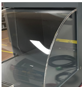
Translucent acrylic protection cylinder with operating handle
