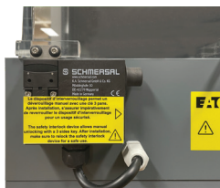
Opening safety system and electromechanical door lock
