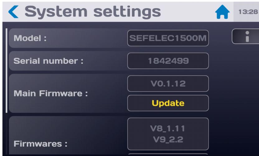
The main HMI firmware file downloaded from our site in 'eaton-maj.zip' format must be copied to the root of a USB stick.
