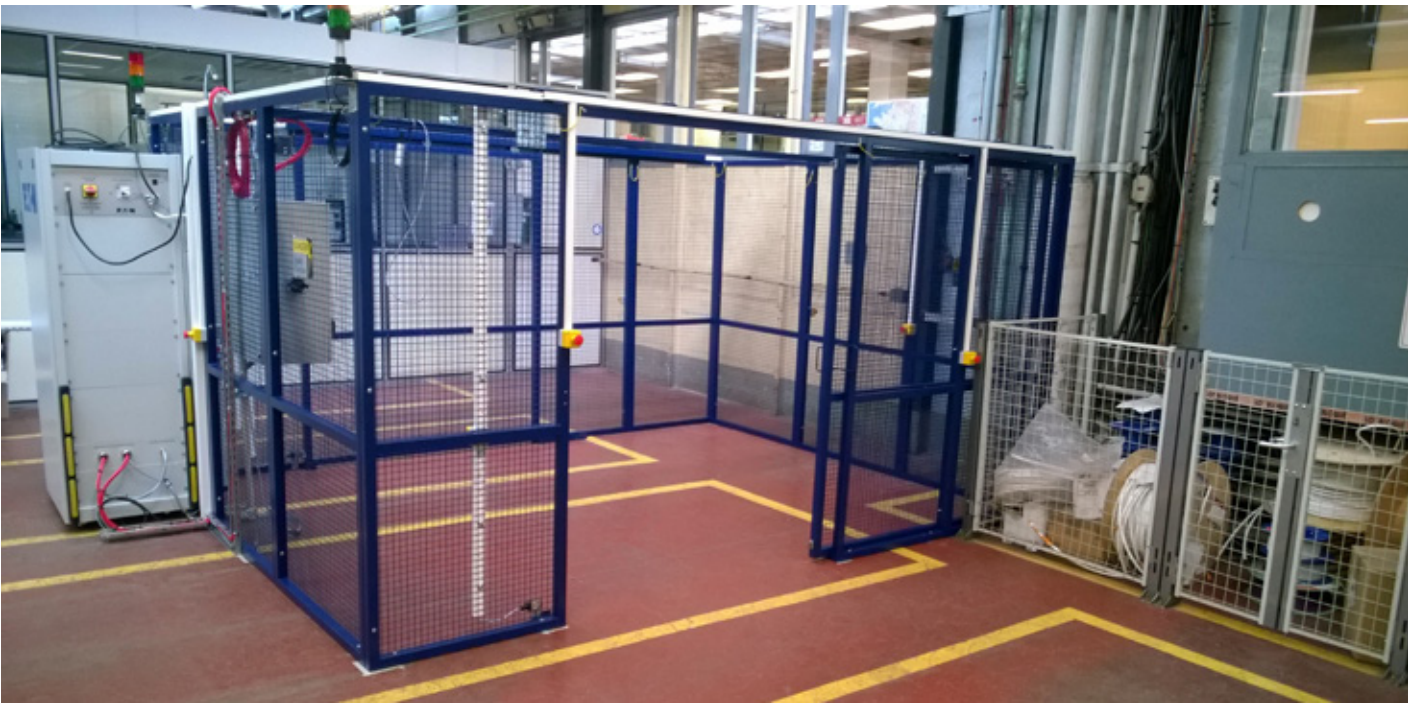
View of the "Go Through" safety enclosure
