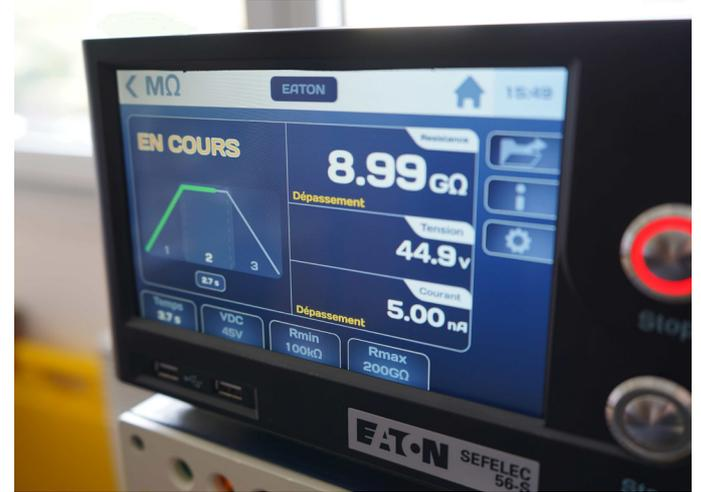
SEFELEC 56-S during an insulation test under 45V
